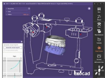
Figure 10: Exported sequential wax-up movement in exocad® Jaw Motion.
