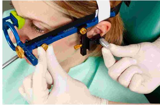
Loosen and remove the porus knobs.
