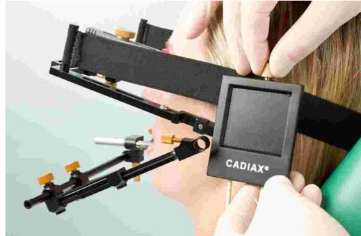
Fixate the styli with the respective screws in the retainers of the lower face bow. The cable of the stylus should hang downwards after it is fixated.
