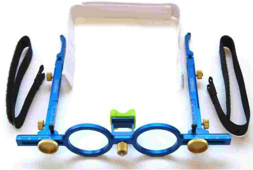
Fixate the glabella support by pushing it from the side into the center position until it snaps in.
