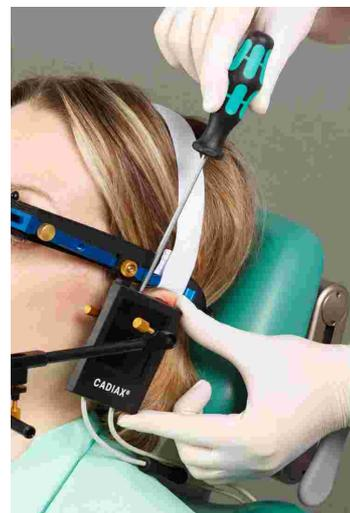
Fixate the styli with the respective screws in the retainers of the lower face bow. The cable of the stylus should hang downwards after it is fixated.
