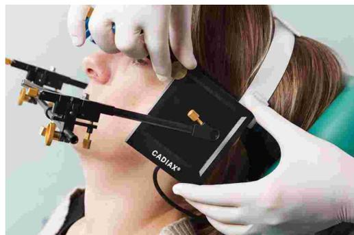
The double-stylus system allows for a recording of the hinge axis rotation on both sides.
